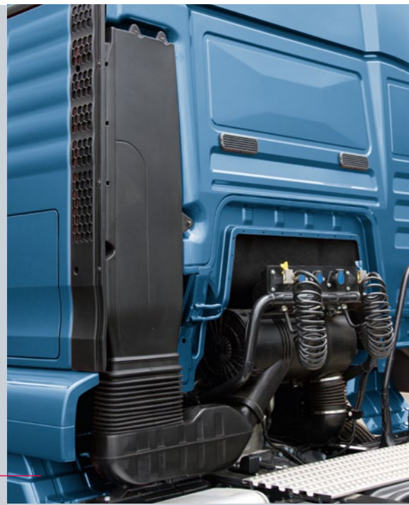
Raised air inlet.
