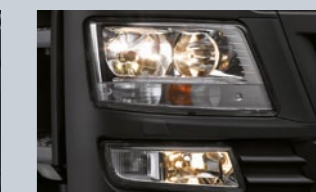
Headlight with free form reflectors.
