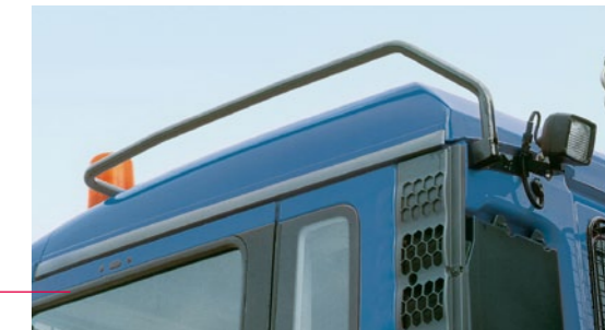
Roof rail on driver's side, and access for building vehicles, driver's side.
