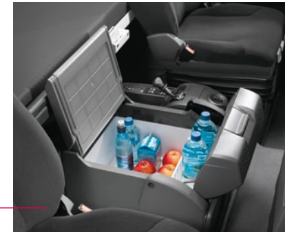
Pull-out insulating or refrigerator box, with fold-out table if required.
