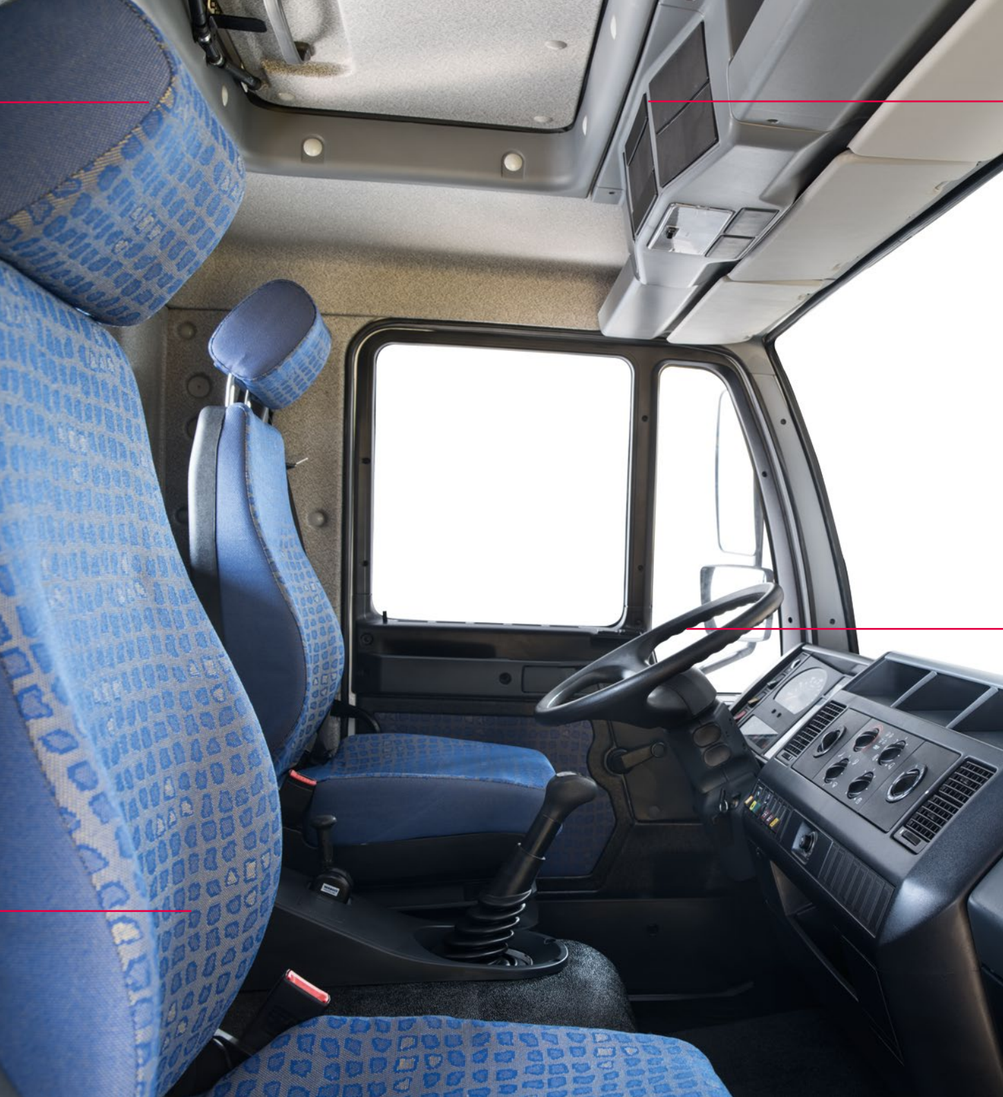
Storage compartments and blank slots for electronic devices such as radio units or tachograph.
