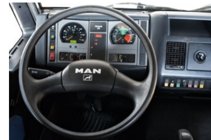
Steering wheel adjustable in height and angle.
